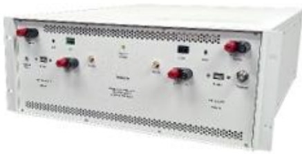
Telebyte 4950 10BASE-T1L Channel Emulator
